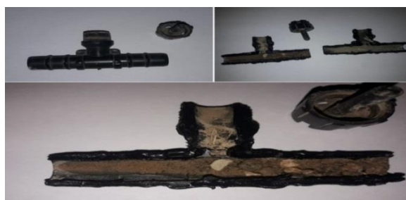
Figure 2. Clogging of droppers and equipment
