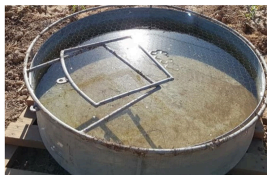
Figure 1- View of the Class A evaporation pan located in the research farm of Lorestan University
