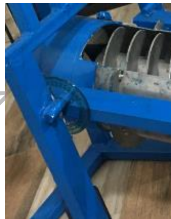
Figure12. Inclination angle measurement.
