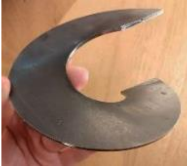
Figure 3. Manufactured blades bent by hydraulic press.
