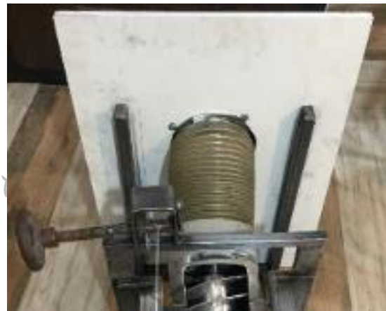
Figure 8. Weir and flexible pipe for water conveyance.
