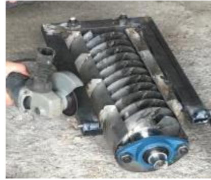
Figure 5. Screw placed in the trough by the bearings.
