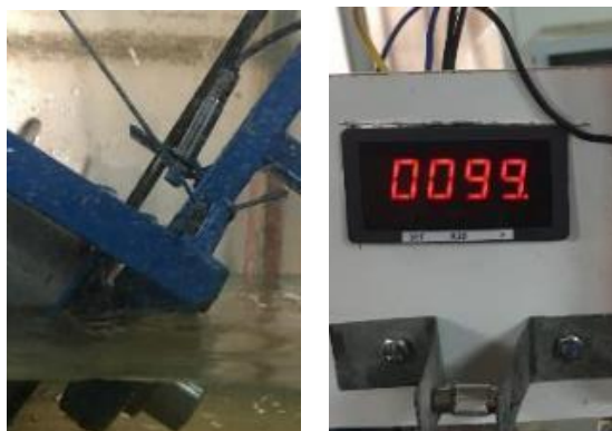
Figure 10. Inductive sensors (left) and digital tachometer (right)
