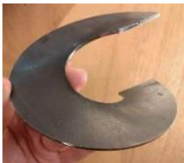
Figure 3. Manufactured blades bent by hydraulic press
