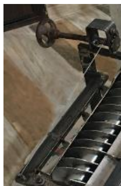
Figure 7. Inclination angle adjustment system
