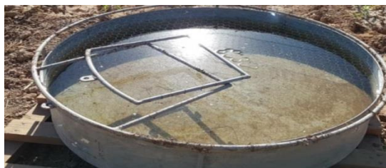
Figure 1. A view of the evaporation pan installed in the field
