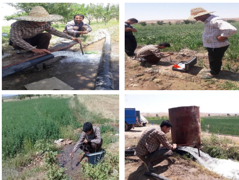
Figure 2. Measuring the inflow discharge in the experimental farms
