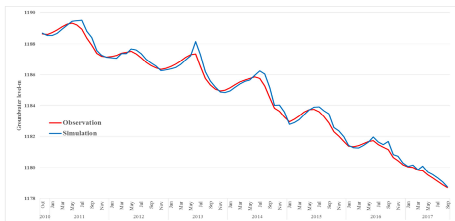
Figure 4. Comparison of the aquifer hydrograph simulation results with the observed data
