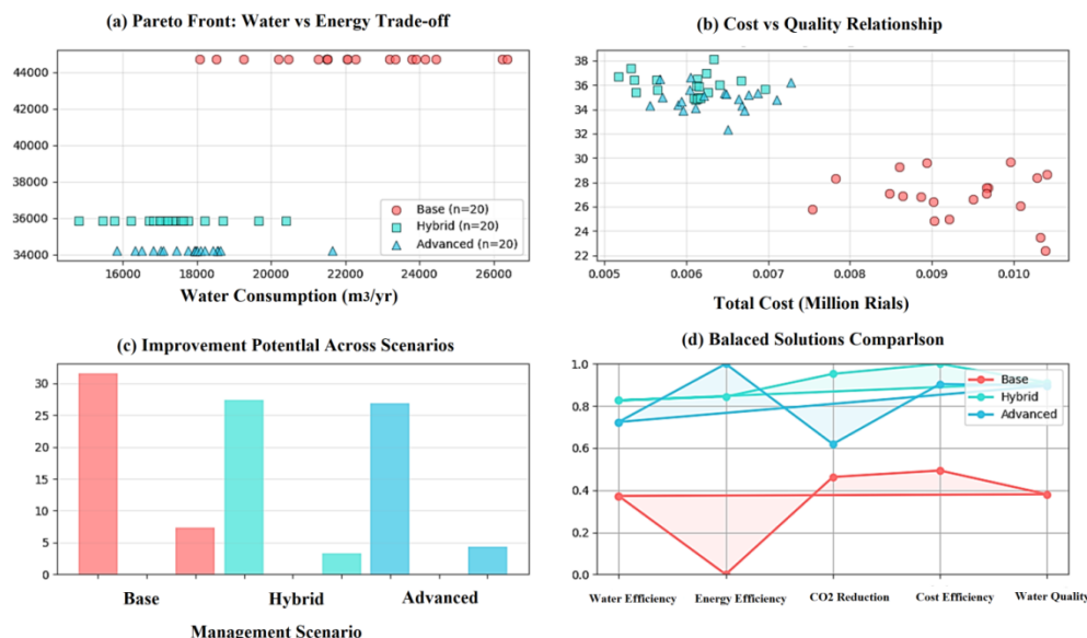
Figure 7. Multi-objective optimization results: (a) Water-Energy Pareto front, (b) Cost vs. Water Quality trade-off, (c) Scenario improvement potential, and (d) Radar chart of integrated WEFЕ performance
