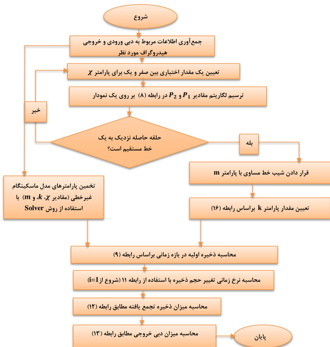
Figure 1. The methodology used in this study for the Muskingum flood routing approach
