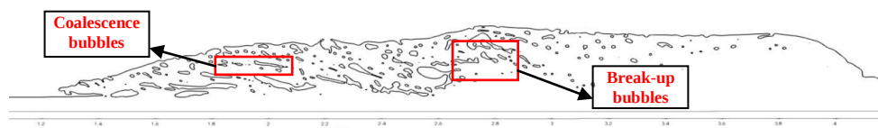
Figure 12. Bubbles in hydraulic jump: numerical (openfoam) image
