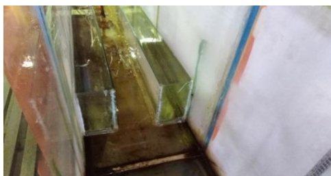
Figure 3. Glass plates installed in the channel
