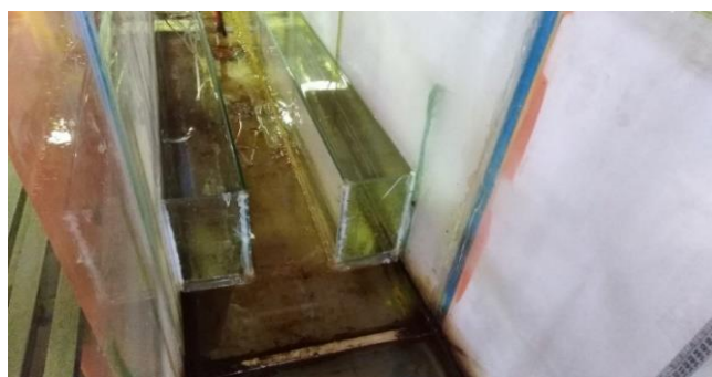
Figure 3. Glass plates installed in the channel
